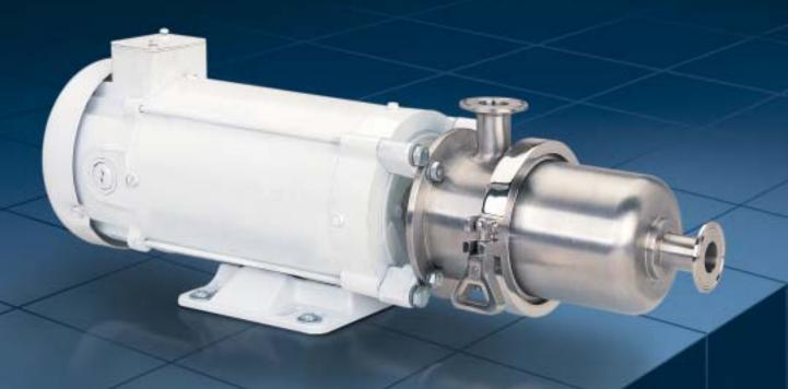
New Moyno® 500 Sanitary Pumps offer low flows and high performance in a compact, cost-effective size. An extension of our popular Moyno Sanitary pump line, versatile Moyno 500 Sanitary Pumps feature 316 stainless steel materials of construction to meet 3A sanitary design standards, as well as elastomers that satisfy FDA requirements. The exclusive Quick Disassembly Clamp makes pump disassembly and cleaning easy, reducing maintenance and labor costs.
